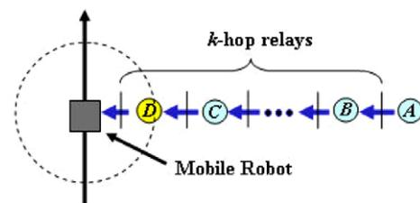
Fig. 1. An example of  $k$ -hop relay mechanism.
