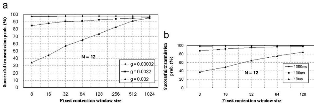
**Fig. 10.** Percentage of successful transmission probability for different size of *fixed contention window* with different packet generation probabilities and fixed node numbers ( $N = 12$ ). (a) Theoretical result. (b) Simulation result.
