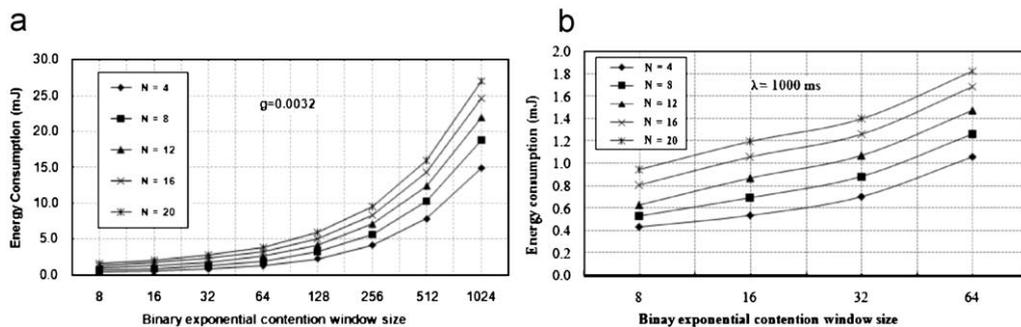
**Fig. 9.** Energy consumption for different size of *binary exponential contention window* with fixed packet generation probability and different node numbers. (a) Theoretical result. (b) Simulation result.
