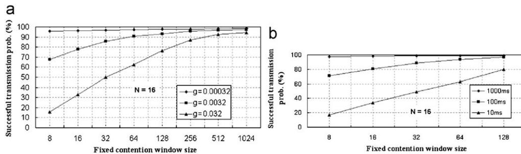
Fig. 12. Percentage of successful transmission probability for different size of fixed contention window with different packet generation probabilities and fixed node numbers ( $N = 16$ ). (a) Theoretical result. (b) Simulation result.
