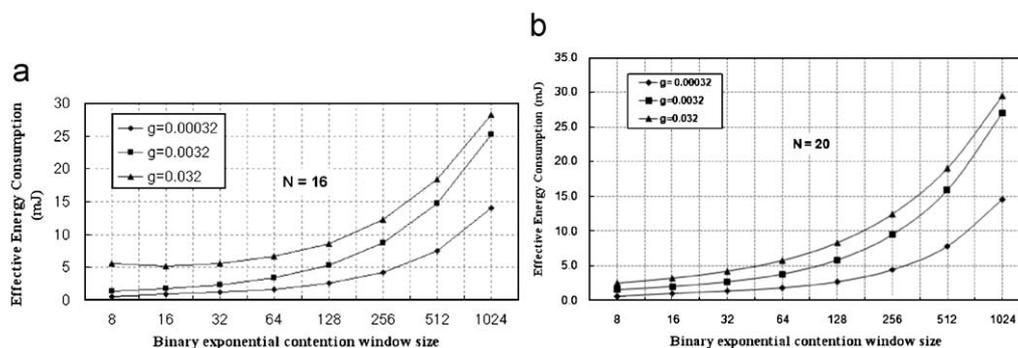
**Fig. 15.** Effective energy consumption vs. *binary exponential contention window* for different packet generation probabilities with fixed number of nodes. (a) Node numbers ( $N$ ) = 16. (b) Node numbers ( $N$ ) = 20.
