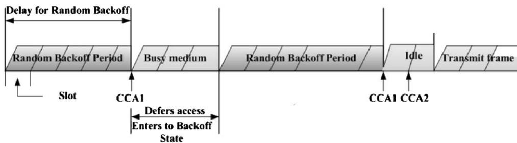
Fig. 1. Basic channel access procedure in our hybrid CSMA-CA mechanism.
