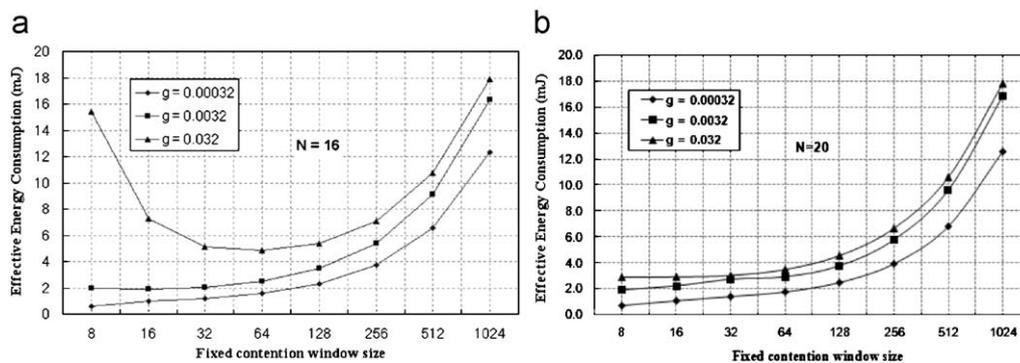
Fig. 14. Effective energy consumption vs. fixed contention window for different packet generation probabilities with fixed number of nodes. (a) Node numbers ( $N$ ) = 16. (b) Node numbers ( $N$ ) = 20.
