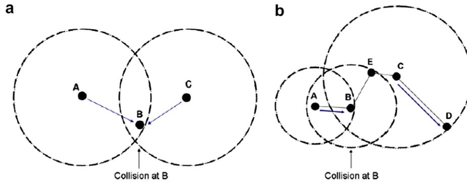
Fig. 1. Hidden terminal problem (a) symmetric case (without RTS/CTS mechanism) and (b) asymmetric case (with RTS/CTS mechanism).
