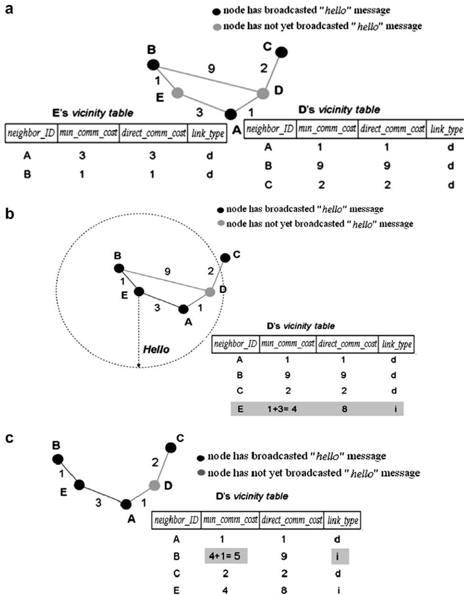
**Fig. 5.** (a) Vicinity tables of nodes D and E, (b) a record of new neighbor E is inserted into D's vicinity table with  $min\_comm\_cost = 4$ , (c) the  $min\_comm\_cost$  from node D to node B is updated to 5.
