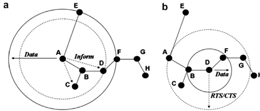
Fig. 6. (a) A broadcasts an “Inform” message to the interfered neighbors C and D and (b) D broadcasts a control packet to inform nodes A and C prior to data transmission.
