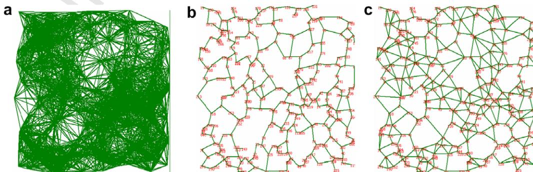
Fig. 7. Network topologies of 100 nodes constructed by (a) without topology control, (b) XTC protocol and (c) LFPC protocol.
