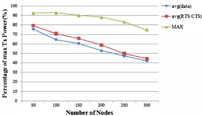
Fig. 12. Percentage of transmission power of data and control packets in the LFTC protocol.
