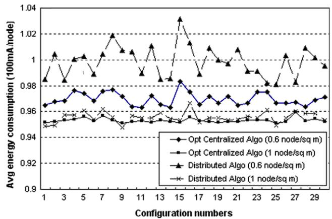
Fig. 8. Average energy consumption for different configurations with different node densities.
