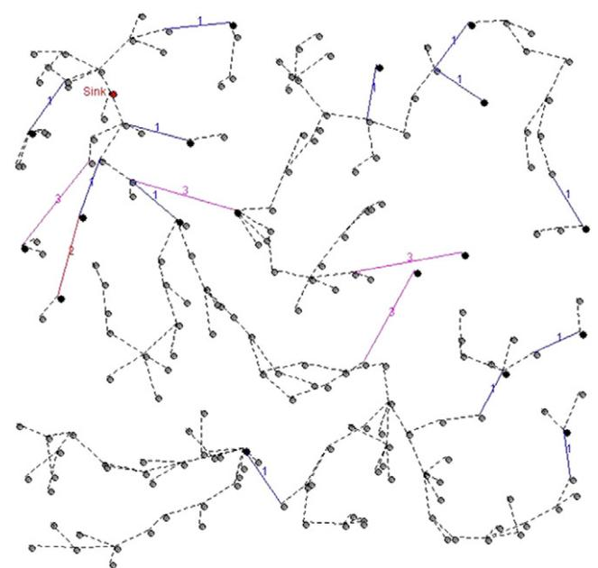
Fig. 14. Configuration of 200 nodes with variable transmission power deployed over 100 m × 100 m area.
