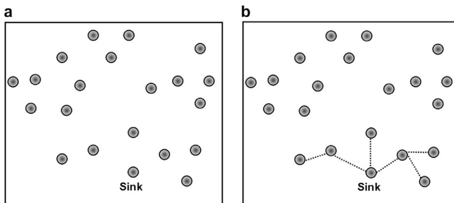
Fig. 4. (a) Randomly distributed sensor nodes over an area. (b) Construction of the first tree topology.
