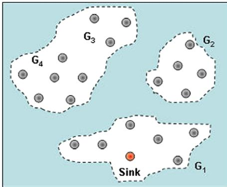
Fig. 1. Randomly deployed sensor nodes with connectivity holes among different group of nodes.
