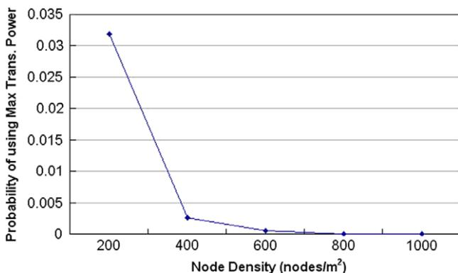
Fig. 12. Probability of using maximum transmission power for various node numbers.
