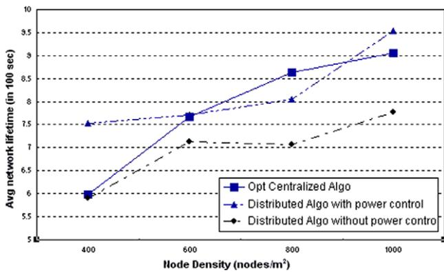
Fig. 10. Average network lifetime for different node numbers with and without power control.
