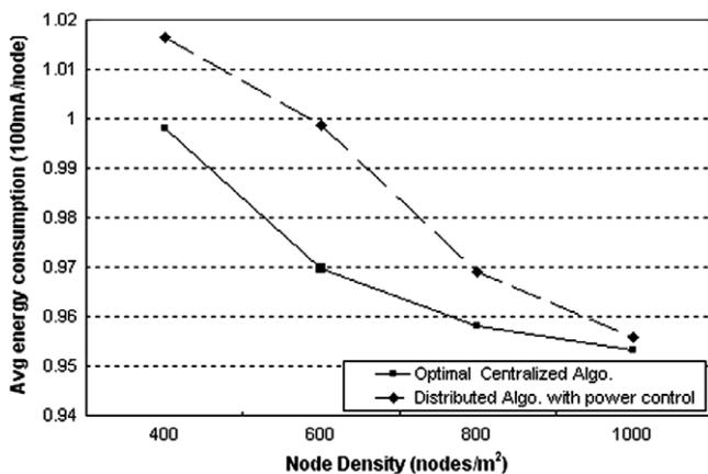
Fig. 7. Average energy consumption for different node densities with transmission power control.
