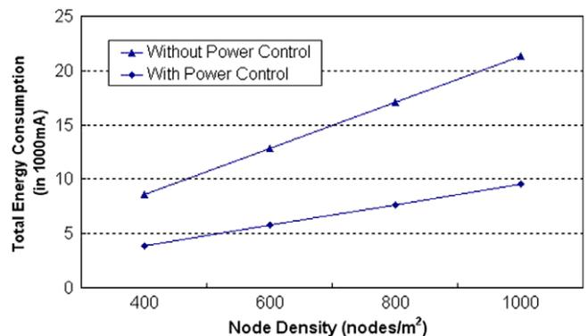
Fig. 9. Total energy consumption for different node densities with and without power control.
