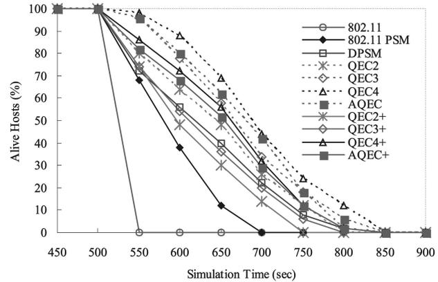
Fig. 9. The effect of different MAC protocols on the fraction of alive hosts with zero workload.
