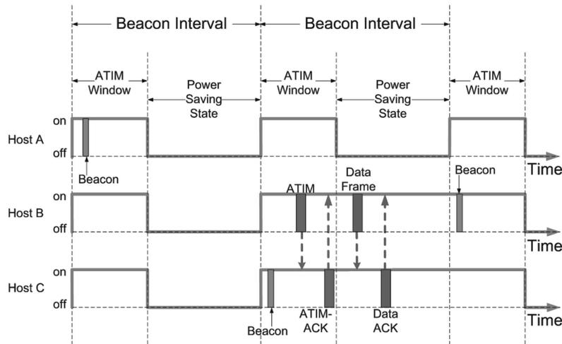
Fig. 1. Power saving mechanism in IEEE 802.11 DCF.
