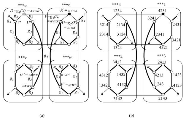
**Fig. 5.** An  $X_4$ -ring on  $S_4$  with faulty node 4231.
