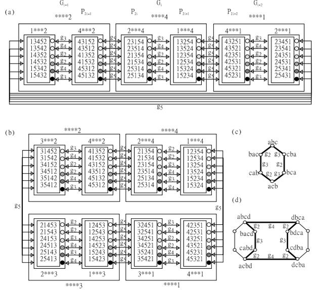
**Fig. 2.** Six pairs of disjoint cycles in (a) a  $(4,3)$ -ring, (b) a  $(4,4)$ -ring, and a distinct cycle in (c) a 3-star and in (d) a 4-star.
