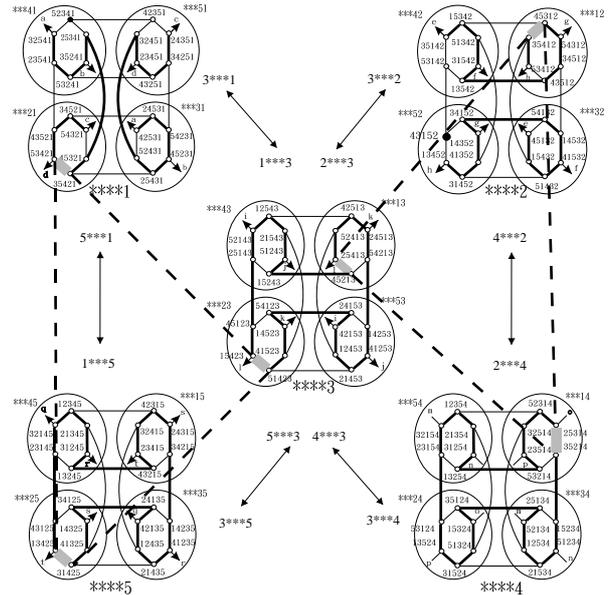
**Fig. 6.** Constructing an  $X_5$ -ring on faulty  $S_5$  with two faults using two  $R_{4,3}$ 's.
