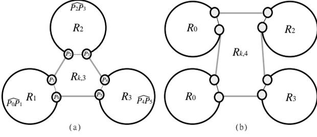
Fig. 3. (a)  $R_{k,3}$  and (b)  $R_{k,4}$  concatenate three and four disjoint rings into larger rings, respectively.
