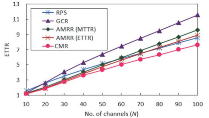
(b) ETTR vs. the number of total channels  $N$ Fig. 6. Performance of MTTR and ETTR with different protocols when  $\theta = 0.7$ ,  $m_1 = 3$ , and  $m_2 = 5$ .
