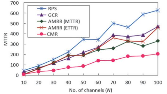
(a) MTTR vs. the number of total channels  $N$
