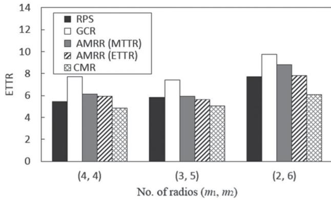
(b) ETTR vs. the number of radios  $m_1$  and  $m_2$ Fig. 7. Performance of MTTR and ETTR with different number of radios  $m_1$  and  $m_2$ .
