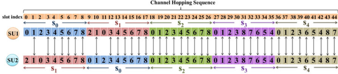
Fig. 4. Rendezvous between two secondary users (SUs) in symmetric synchronous environment.
