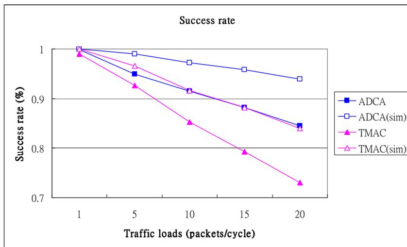
Fig. 14: The average packet transmission success rate for the end-to-end scenario
