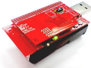
Fig. 6: Octopus II sensor node
