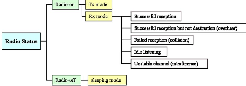
Fig. 5: The radio status of a sensor node
