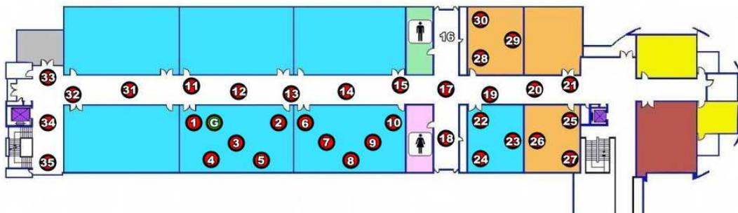
Fig. 7: The deployment of WSNTB sensor nodes
