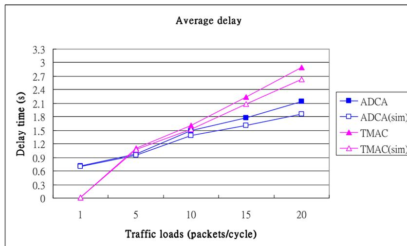
Fig. 11: The average transmission delay for the all-to-one scenario
