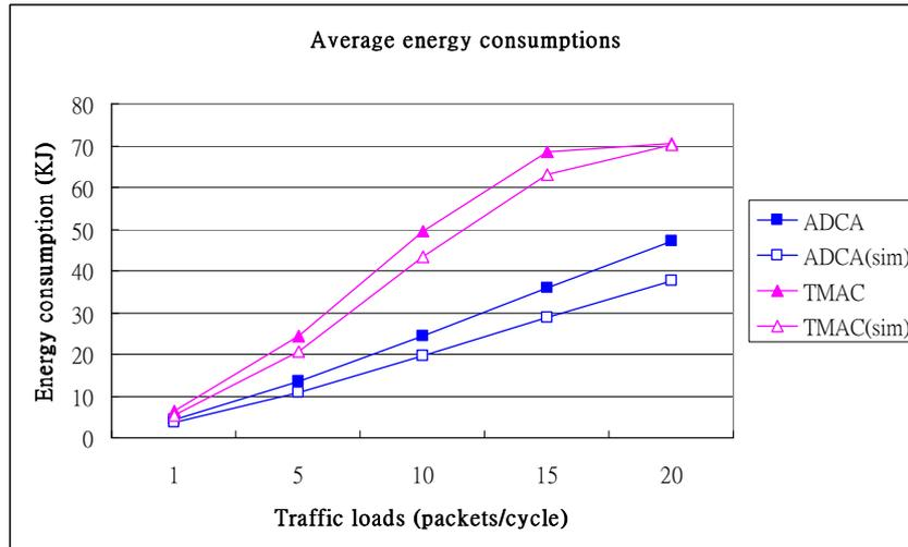
Fig. 10: The average energy consumption for the end-to-end scenario
