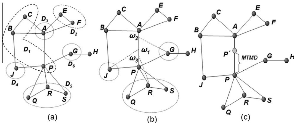
Fig. 4. (a)  $D_1$  and  $D_2$  are DTSs of node *A* and are represented by the dotted curves.  $D_3, D_4, D_5$  and  $D_6$  are the DTSs of *P* and are represented by the solid curves. (b) Taking *A* as a sender and *P* as a receiver, shortest distance from each head nodes of *P* is estimated without taking sender *A*. (c)  $PP'$  is the required *MTMD* of *P*. If *A* is dead, each of its head nodes can be connected with it.  $P'$  is the new position of *P* after mobility.
