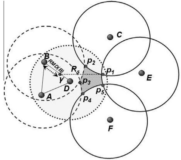
**Fig. 9.**  $p_1$  is the farthest critical sensing point of node  $D$ . In order to estimate  $RMD(B)$ , find a point  $\gamma$  on  $\overline{BD}$  from  $p_1$  such that  $\overline{p_1\gamma} = R_s$ . Hence,  $RMD$  of node  $B$  is  $\overline{\gamma B}$ .
