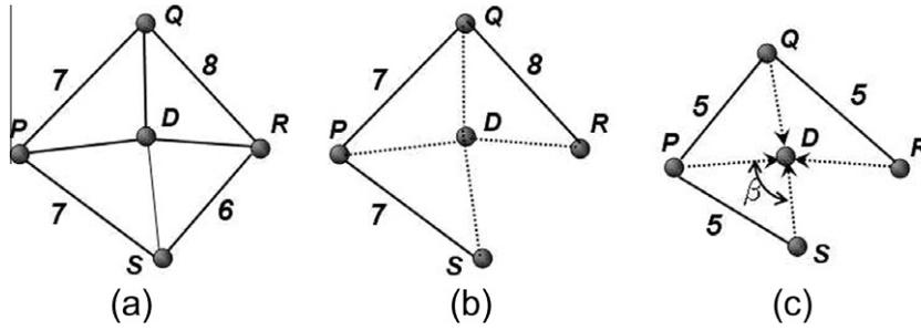
**Fig. 6.** (a) Head nodes form a weighted graph with dead node  $D$ . The weights represent the physical distance between any two nodes. (b) Head nodes  $P, Q, R$  and  $S$  construct the minimum spanning tree. (c) Head nodes  $P, Q, R$  and  $S$  move towards the dead node  $D$  such that the edges of minimum spanning tree is reduced to  $R_c$ , where  $R_c$  is 5 units taken in the example.
