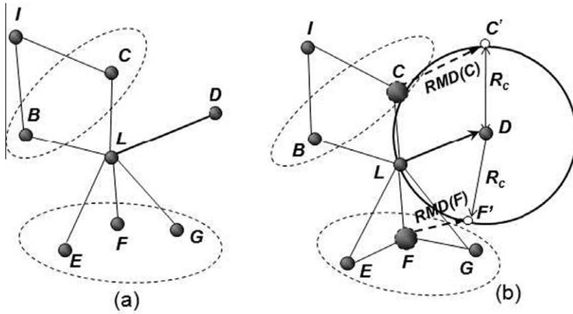
**Fig. 7.** (a) Disjoint Transmission Sets of leader node  $L$ , among its connecting neighbors.  $L$  has to move to the position of the dead node  $D$ . (b) Node  $F$  and  $C$  are head nodes in different DTS of leader node  $L$ . Hence, both  $F$  and  $C$  move parallel to the mobility direction of  $L$  with  $RMD(F)$  and  $RMD(C)$  units, respectively, so that the connectivity between  $F$  and  $L$  and  $C$  and  $L$  is not lost.
