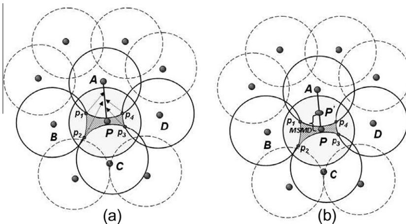
**Fig. 5.** (a) Here, the shaded region is one-covered and death of node  $P$  creates the coverage problem. Hence,  $P$  estimates its *MSMD* with respect to its CSPs. (b)  $P$  estimates its *MSMD* as  $PP'$  so that its mobility from  $P$  to  $P'$  does not affect the existing coverage.
