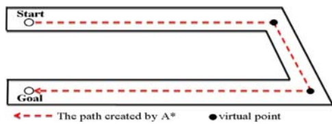
Figure 10 A path from start to goal with virtual points (see online version for colours)
