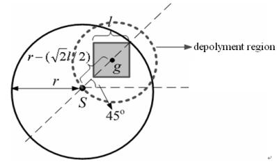
Fig. 5 The dashed circle is a simplified deployment region with respect to grid  $g$ .
