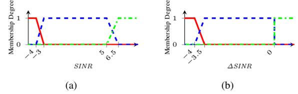
Fig. 4: The membership functions (a)  $\mu_B(SINR)$ ,  $\mu_M(SINR)$ , and  $\mu_G(SINR)$ , and (b)  $\mu_P(\Delta SINR)$ ,  $\mu_F(\Delta SINR)$ , and  $\mu_N(\Delta SINR)$  shown in red solid, blue dashed, and green dashdotted lines, respectively, where  $\mu_F(\Delta SINR) = 0$  and  $\mu_N(\Delta SINR) = 1$  if  $\Delta SINR = 0$ .
