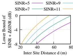
Fig. 6: The impact of the inter site distance of small base stations on  $SINR + \Delta SINR$  for  $SINR = 5, 7, 9, 11$ .
