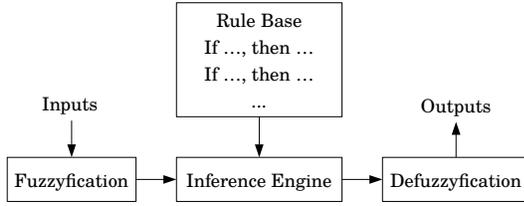
Fig. 3: The architecture of a fuzzy logic system.
