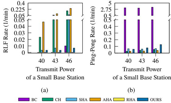
Fig. 8: Impact of the transmit power of the small base station on the (a) RLF rate, and (b) ping-pong rate when the average number of small base stations per macro base station is 30.
