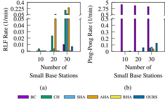
Fig. 7: Impact of the average number of small base stations per macro base station on the (a) RLF rate, and (b) ping-pong rate.
